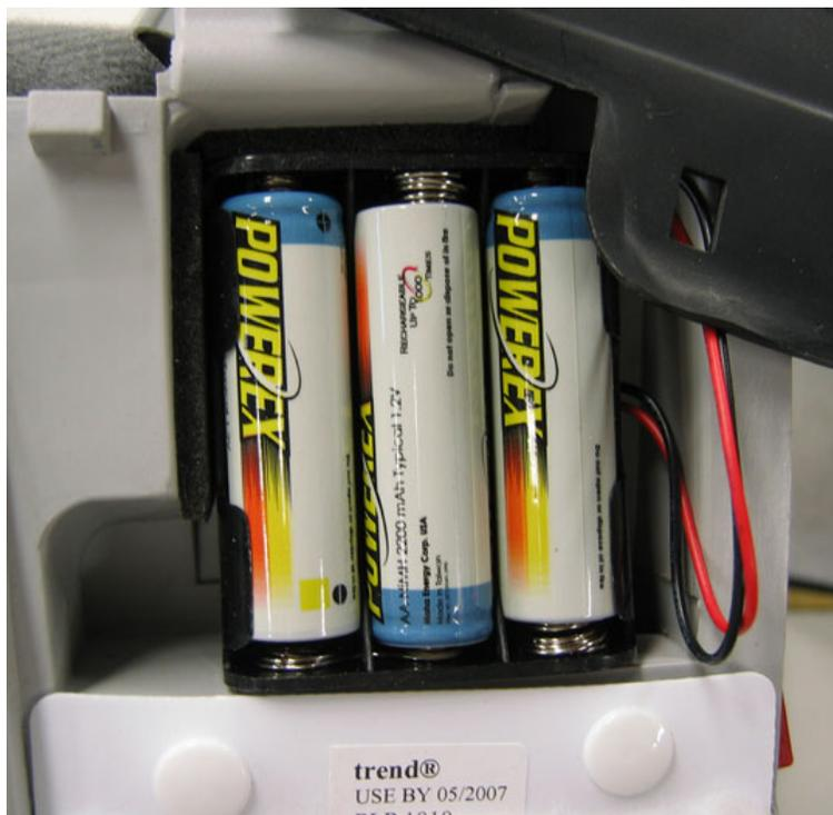
Here is the poor fit of the original battery pack:
