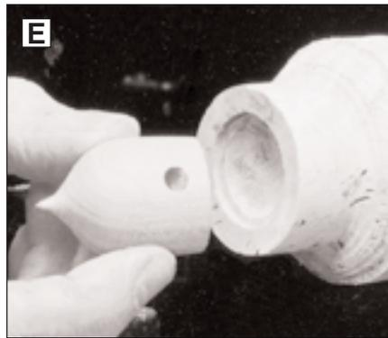
Prior to refining the rest of the birdhouse cap, check the fit of the cap to the body of the birdhouse ornament.
