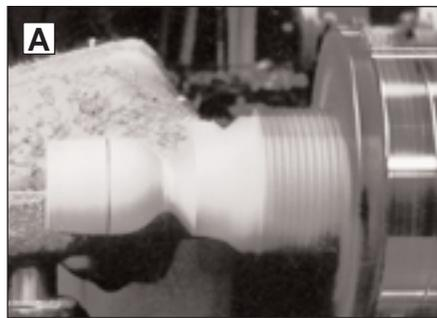
Turn the body of the acorn birdhouse, leaving sufficient material at the base for hollowing. Note the pencil line at the opening for the perch; it should be untouched.
