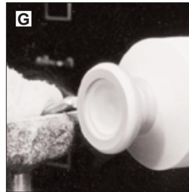
Once the fit to the cap is snug, use a spindle gouge to refine the shape of the acorn cap.
