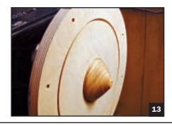
When the chuck is fully tightened, you can turn the bottom. I usually leave the tailstock in place as long as possible for safety, but it can be removed for completing the bottom. I always use this chuck at a fairly low speed – perhaps 600 or 800 rpm at maximum.
