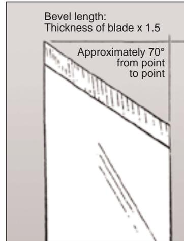
Typical grinding of a skew chisel
