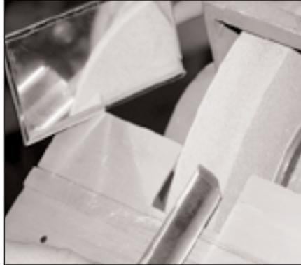
Until you have a sense of where you are grinding on the tool, it's helpful to either place your head to the side of the wheel or make use of a small mirror. The mirror, shown above, allows you to see your placement of the tool on the wheel.
