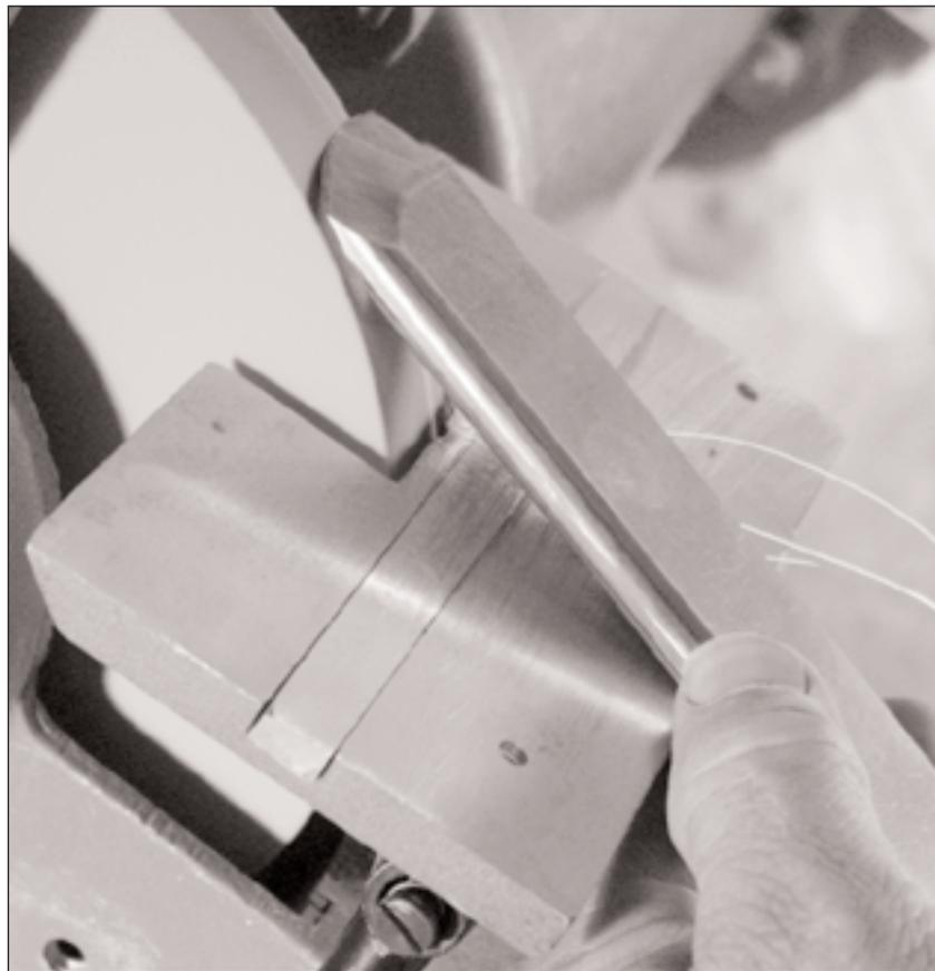
Using the back edge of the tool rest, pivot the curved skew to grind the edge. Use rotational movement, grind in the area that is roughly parallel to the face of the wheel.
