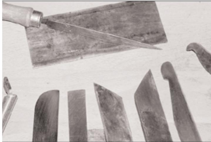
Turning scrapers are quite similar to the cabinetmaker's scrapers (shown with a burnisher). Both types of scrapers usually cut with a burr and make use of a burnisher to raise that burr. Turning scrapers are thinner in weight and come (or can be made into) in an array of shapes for various uses.
