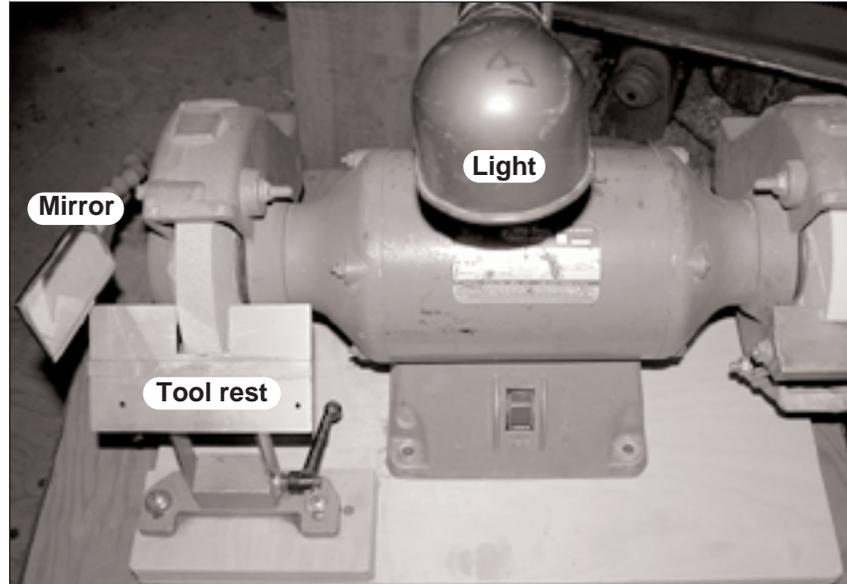
Strong and sturdy tools rests, good lighting, solid mounting and at least one good wheel are minimal requirements for a reliable grinder. The tool rest on the left is an after-market rest. A supporting strap was added to the right rest for increased rigidity.
