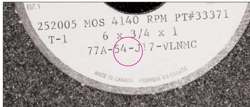
It is challenging to look at a wheel and guess its grit size and hardness. Most stones have a code—in this case, the bottom row of numbers. The most important code for a turner are circled. The "54" designates grit size; "J" indicates the hardness designation.
