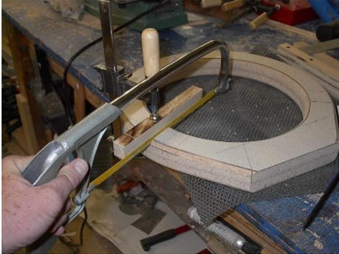
Clamp a short piece of hardwood to the layout line on one side of the slot. Use it as a guide to make the kerf straight and use a hacksaw to cut just below your depth mark. Repeat this 5 times and you'll have nice straight sides for the slots.
