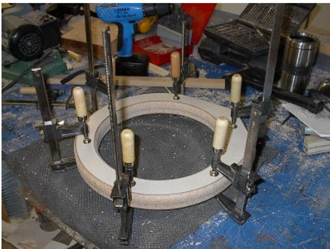
Before starting to glue up the 2 pieces, try sanding to the lines to make them matching pairs as close as possible. Once the interior and exterior are pre-sanded, glue them together to dry over night. Remove the clamps and do the finish sanding on the exterior and interior. Once sanded, use a round-over bit in your router and clean up all the edges, but NOT the bottom edge that sits on the lathe
