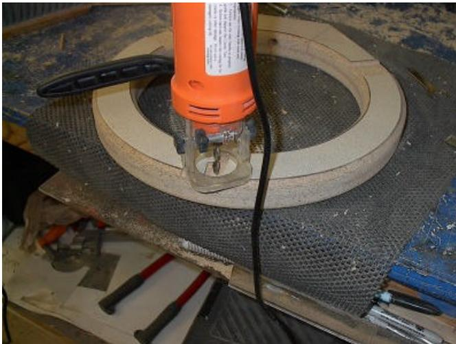
I cut out the slots with a cut-out router Roto-Zip or similar (Harbor Freight \$19.95)  $\frac{1}{4}$ " deep but any router would work as long as you have a see through base. Be careful not to touch the nice straight kerfs you took so much time to produce. Clean up the slots with a sharp chisel.
