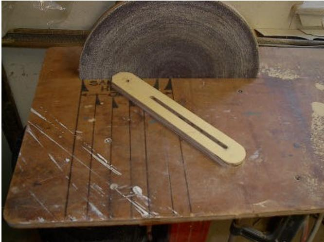
Round and smooth the ends of each roller arm and the side of each roller arm to fit the slots you cut in the main body of the steady rest. Since each slot will be slightly different in width, mark each arm and their respective slots and sand the edges to fit.
