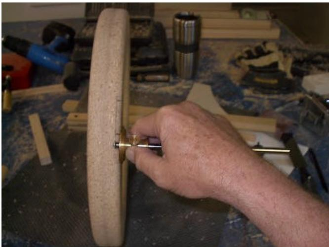
Mark out the slots for the roller arms using a marking gauge, darken the gauge lines with a pencil. The roller arms are ½" MDO (medium density over-lay) material used by the venerable "Norm" in many of his projects. It's used almost exclusively by the sign industry. Any sign supply house can sell you a sheet. (Can you guess what I did in a former life?)
