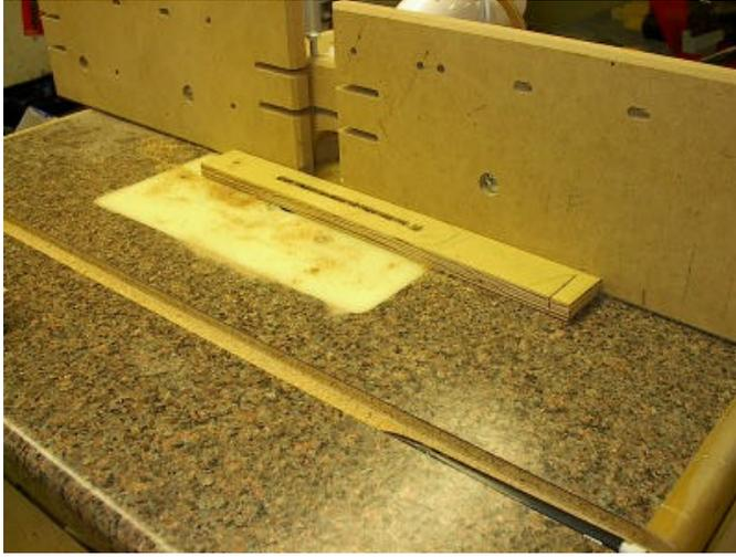
Rout the slots in the roller arms using a 1/4" router bit. Set the depth of the cut to be just a "smidge" more than half way. Then turn the arm over and rout through the other side. Drill the 1/4" hole for the roller bolt.
