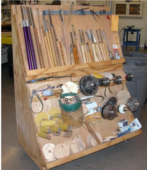
We used to have a big, wheeled cart that held all the tools, but its base was 48 inches by 36 inches, and it took up way too much floor space. As you can see, more space is wasted than is used. It was not an efficient design, by any standard.
