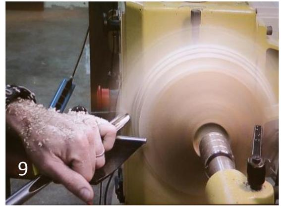
**Hints:** Always sharpen your gouge before making the final cuts on the thin wings. It will give you a cleaner cut and will take less force to make the cut, thereby putting less pressure on the wing.
