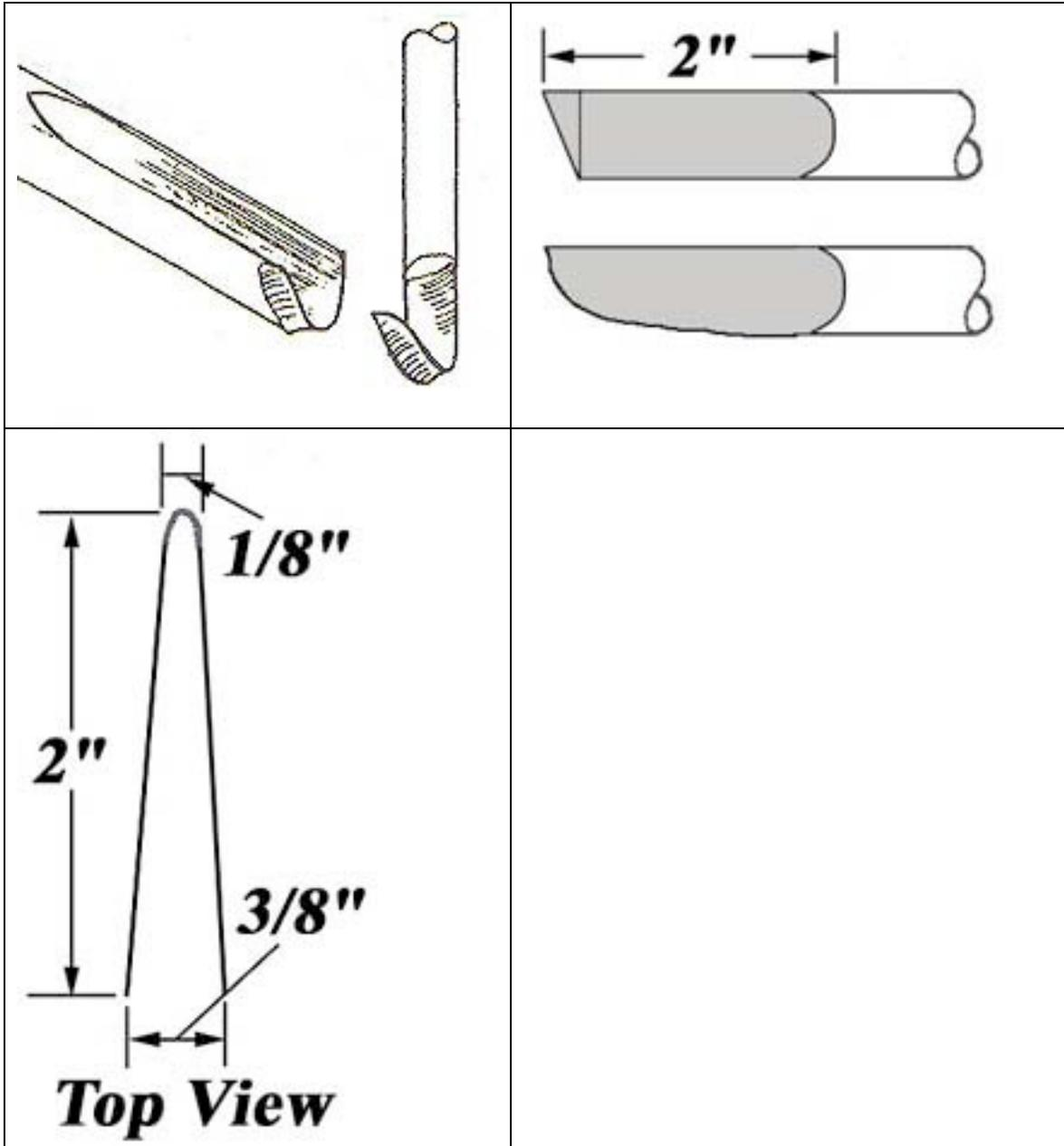
**Step 1:** Cut the drill rod with a hacksaw to 9" lengths. Process to grind one end to the example shown. You can do this with a wheel grinder, but a belt type grinder is easier and leaves a better finish. Determine the cutting edge side, but don't get it sharp at this point. With the cutting edge down, file the left face to a clean flat face—as this will be the inside flute of your hook tool.
