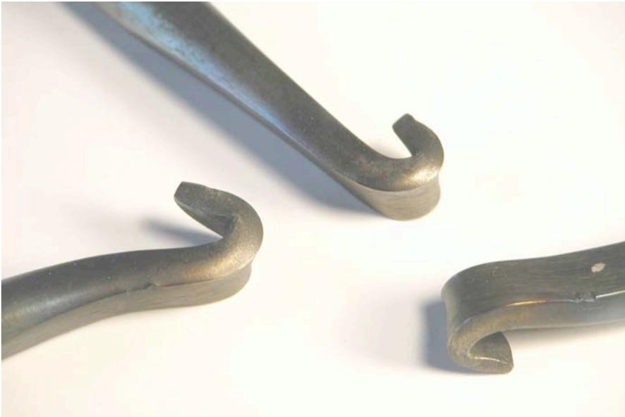
**After hardening the steel, heat well back of the hook and allow conduction to bring the bronze color up to the hook area. When it appears an even bronze quench quickly into water to halt the process.**
