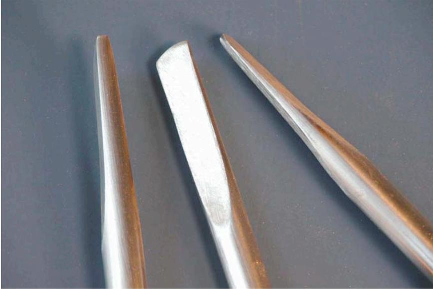
**Grind the blank into this shape. Left: the view from above. Center: left face (cutting edge down). Right: what will become the cutting edge.**
