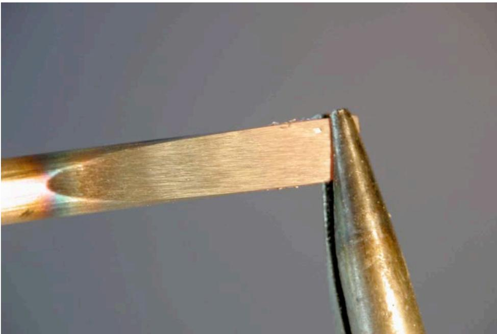
**Grip the bright cherry red end of the blank with the needle nose pliers and bend into a hook--grip near the end to produce a smaller hook. If the cutting edge is facing downward, bend the hook to the left.**
