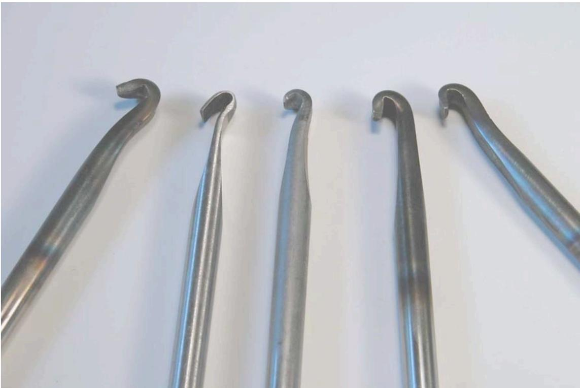
**Experiment with hook shapes, sizes and off-sets. For your first hook do a simple straight tool with no off-set.**
